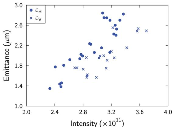
Figure 4: Transverse emittances in the Q20 optics.
