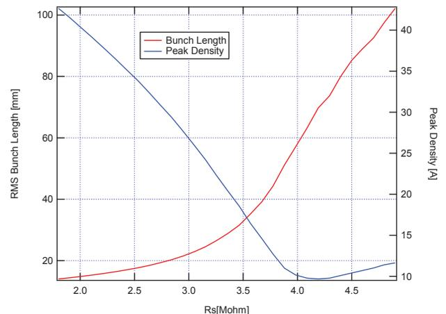
Figure 3: RMS bunch length and peak bunch density as a function of HC shunt impedance for a fixed HC detuning of -56.5 kHz.
