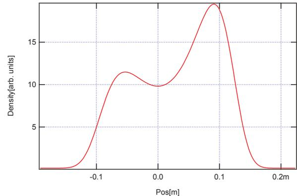
Figure 2: Fully self-consistent equilibrium density distribution for  $R_s = 4.2$  M $\Omega$ , HC detuning = -56.5 kHz. The RMS bunch length is 69 mm. Other parameters are the same as in Figure 1.
