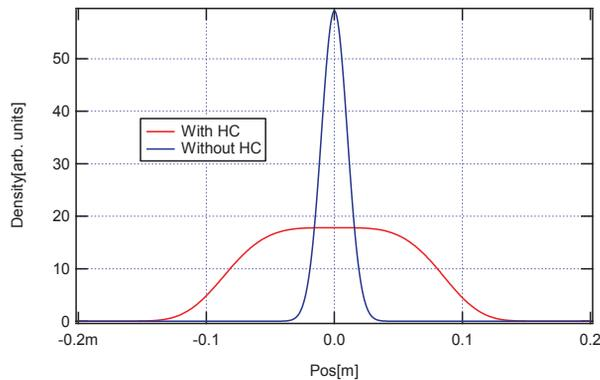
Figure 1: Equilibrium (scalar self-consistency) bunch density distribution for  $R_s = 2.017$  M $\Omega$ , HC detuning = -28.4 kHz ( $Q=21600$ ). The RMS bunch length is 54 mm. Energy loss per turn = 856 keV (machine loaded with 19 IDs). Main cavity voltage = 1.63 MV. For comparison, the distribution with no HC present is also shown, corresponding to an RMS bunch length of 10.12 mm.
