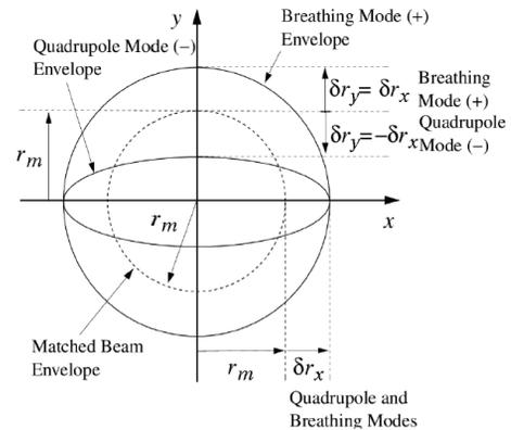
Figure 1: Transverse picture of the envelope modes [4].
