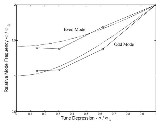
Figure 2: Relative envelope mode frequencies as a function of the tune depression for UMER operating parameters, plotted next to a calculation for the smooth approximation (dashed lines) shown in Eq. 2,3.
