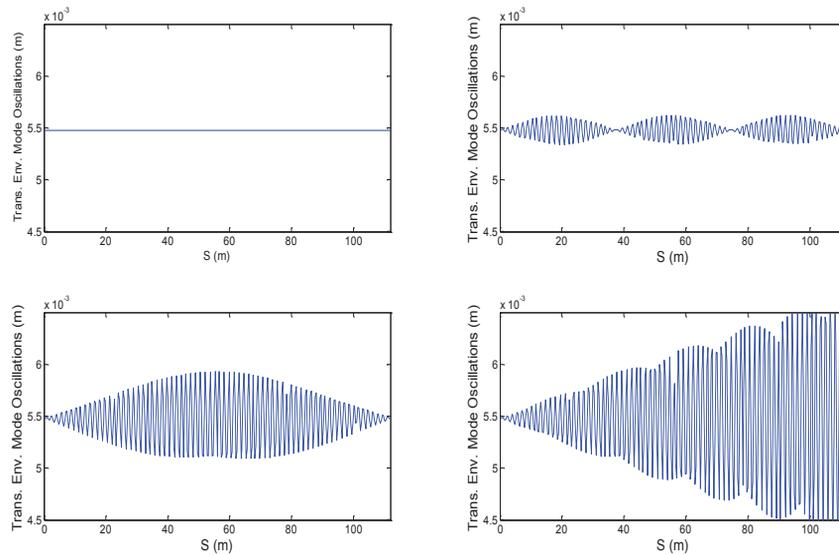
Figure 3: WARP envelope code simulations of the transverse envelope displacement near the quadrupole mode resonance sampled once per betatron frequency. Beam is kicked once per lattice period off resonance (top left), close to resonance (top right, bottom left), and on resonance (bottom right) for 10 turns.
