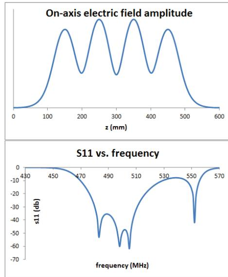
Figure 5: On-axis electric field amplitude and  $s_{11}$  with a tuned coupler.
