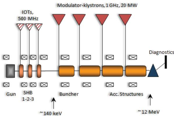
Figure 1: CLIC drive beam front-end layout.
