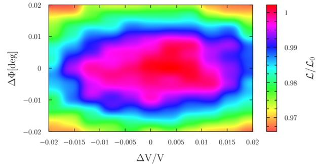
Figure 5: Crab Cavity phase offset and voltage tolerances.
