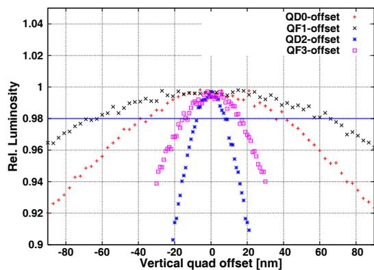
Figure 3: Vertical quadrupole offsets versus relative peak luminosity for the last four quadrupoles with IP feedback.
