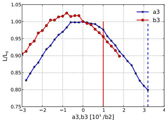
Figure 4: Luminosity loss due to sextupolar components in QD0.  $a_3$  in blue (dashed),  $b_3$  in red (solid). Values are given as relative to  $b_2$  divided by  $10^4$ , for a radius of 1 mm. The vertical lines show the measured values in the prototype.
