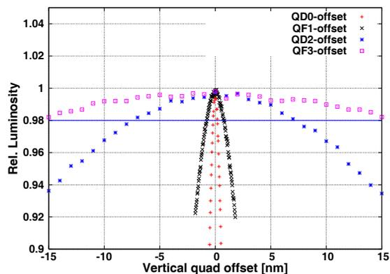
Figure 2: Vertical quadrupole offsets versus relative peak luminosity for the last four quadrupoles.
