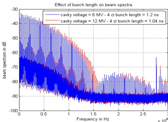
Figure 2: Effect of reducing bunch length on measured LHC beam spectrum (in dB) from 1.2 ns (in blue) to 1.04 ns (in red). The first notch of the distribution is observed to shift from 1.5 GHz to 1.7 GHz. The peaks beyond 2.7 GHz are believed to be due to the acquisition system bandwidth.
