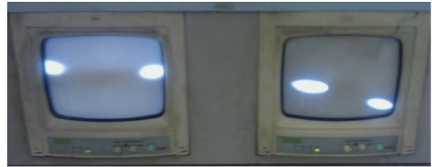
Figure 6: SR images of the 1.1 mA electron (left) and the 0.3 mA positron (right) bunches on the TV monitors while applying the RF separation at the 6.5 kV peak voltage. Electrostatic separation system is fully off.
