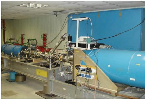
Figure 2: General view of the commissioned first acceleration station of the JINR electron linac.
