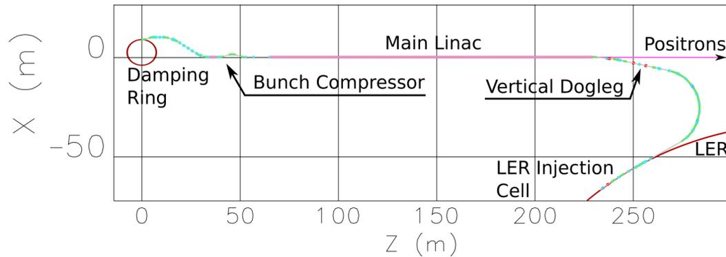
Figure 2: Layout of the electron injector from the DR extraction to the LER injection cell.
