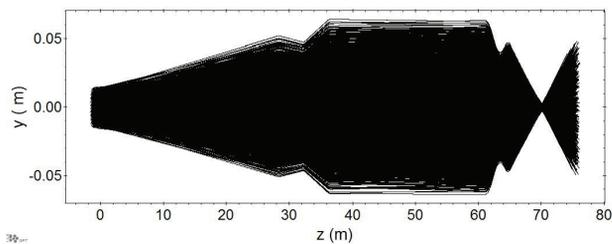
Figure 8: Vertical beam trajectories in the final focus.
