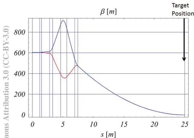
Figure 5: Final focus system with a large gap between the last quad and the target, and  $\beta^* = 0.6$  m.
