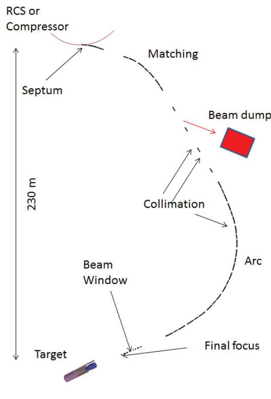
Figure 2: Layout of the proton-beam transport at a Neutrino Factory.
