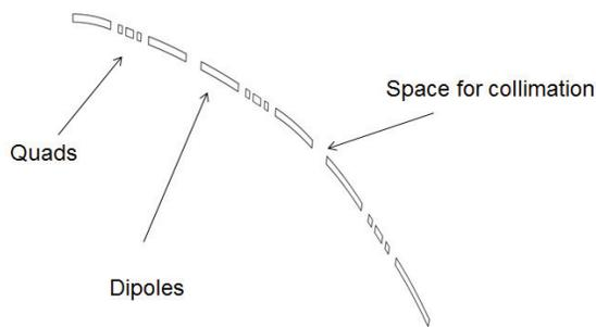
Figure 3: Several cells of the arc lattice.
