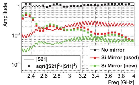
Figure 7: S-Band transmission measurement of a used and a new silicon bulk-dielectric coated mirrors, compared to the same measurement on an empty cavity.
