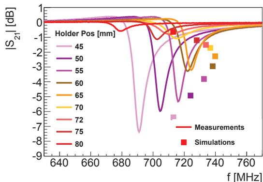
Figure 6: Resonance vs. horizontal mirror holder position, as measured and simulated with the stretched wire method.
