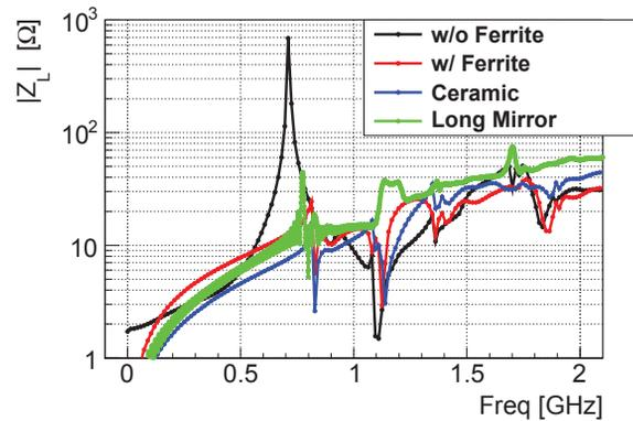
Figure 3: Comparison of different mirror support configurations (with logarithmic scale of the wake impedance).
