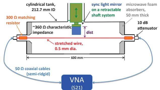
Figure 4: Stretched wire measurement setup.
