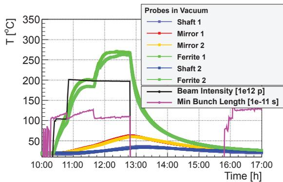
Figure 2: Thermal behavior of the BSRT structure as measured by 5 temperature probes located at strategic location in the vacuum tank, during a dedicated test with high beam intensity and variable bunch length.
