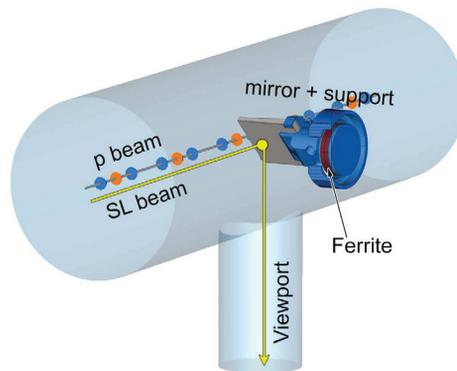
Figure 1: Mirror support system of the LHC synchrotron light monitor.
