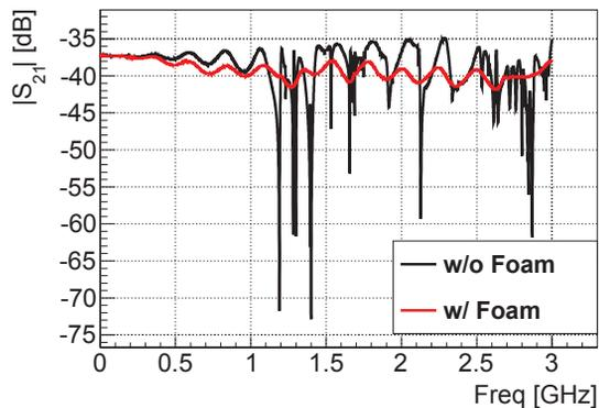
Figure 5: Damping of the parasitic modes in the stretched wire setup by microwave absorbing foam.
