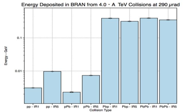
Figure 9: Comparison of the amount of energy deposited in the detector with *p-p*, *p-Pb*, *Pb-p* and *Pb-Pb* collisions.
