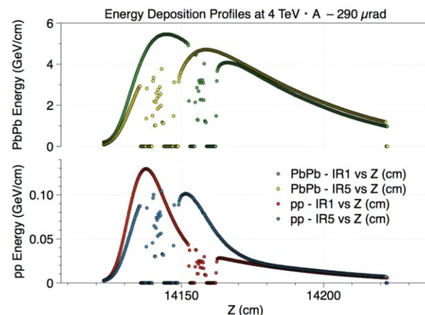
Figure 8: Energy deposited in the TAN for *p-p* and *Pb-Pb* collisions. The region in the center for each detector is where the BRAN is located. The different material in from of the BRAN produces the difference between the shower depositions between the IR regions.
