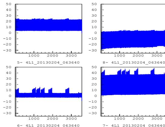
Figure 6: Pulse height mode in ATLAS in *p-Pb* operation. The plot is taken on the detector at the Left side of the IP which captures the shower from the Proton beams.
