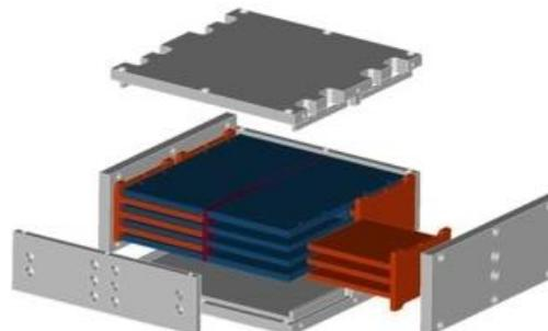
Figure 1: Exploded view of the detector.
