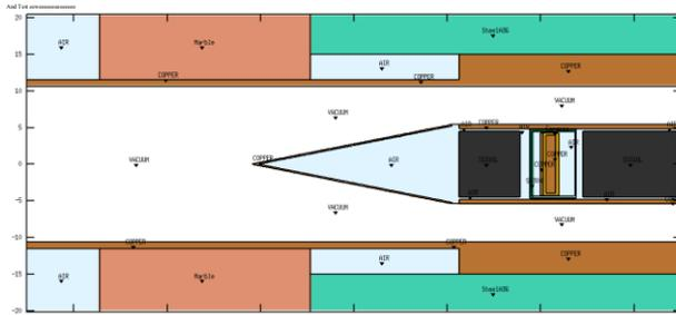
Figure 7: Top view of the BRAN in the CMS TAN. The color white indicates the regions of vacuum.
