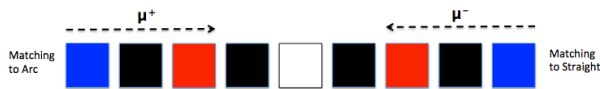
Figure 1: Insertion section schematic. The black rectangles represent triplet magnets while the red and blue rectangles represent kicker magnets and septa, respectively. The empty long drift is shown as a white rectangle.
