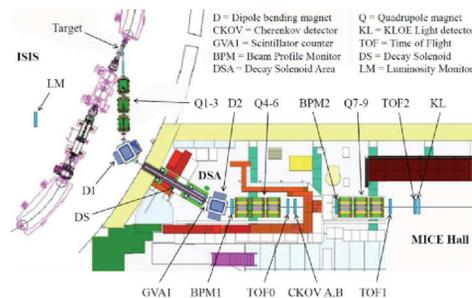
Figure 3: Layout of the MICE beam-line at ISIS.
