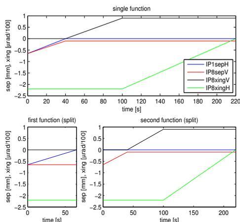
Figure 2: Functions describing the collapsing of separation bumps and changes of crossing angles in adjust. Top: initial function used in 2012; bottom: split functions.
