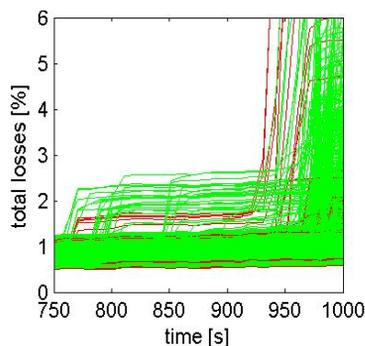
Figure 1: Percent losses per bunch for beam 2 in fill 2731 (time since the start of squeeze): some bunches go unstable and lose intensity non negligibly. Red curves for bunches colliding in IP1/5, green for bunches colliding in IP1/5/8.
