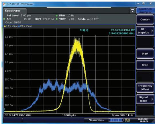
Figure 2: A longitudinal Schottky spectrum of the 3 GeV/u deuteron beam at 3500th harmonics of the revolution frequency, showing the initial spectrum (blue curve) and after 8 minutes of cooling (yellow curve). The beam intensity is  $2 \times 10^9$  ions.
