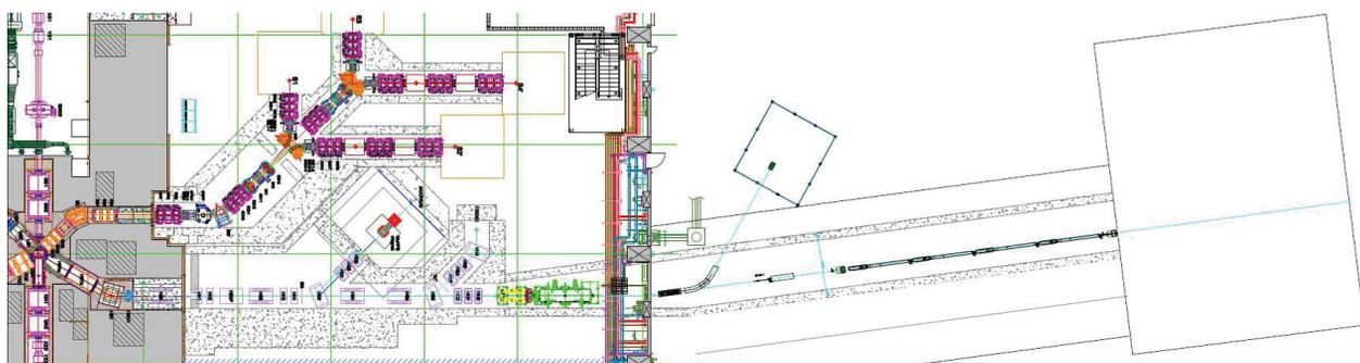
Figure 1: Top view of the muon production target and associated beam transport lines (J-PARC MLF). Two of these secondary beamlines are extracted at the angle of 60 degrees to the proton beamline (forward), and the others are at 135 degrees (backward).
