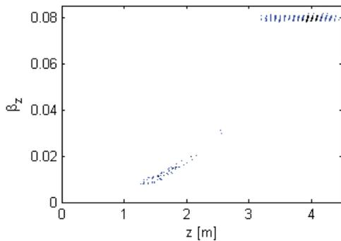
Figure 5: RFQ bunching and acceleration of the beam.
