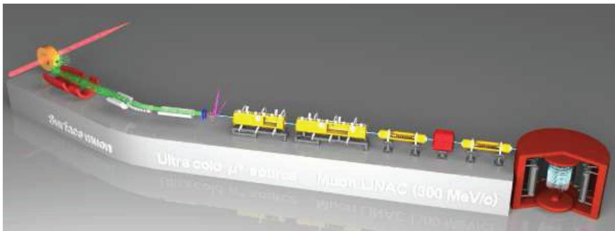
Figure 3: Design of muon linear accelerator.
