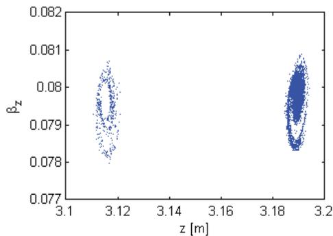
Figure 6: Accelerated bunches of the beam at RFQ output.
