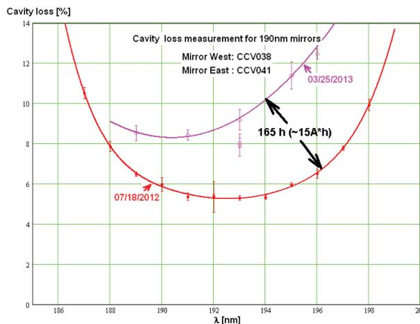
Figure 5: Degradation of VUV 190 nm mirrors during  $E_\gamma=87$  MeV  $\gamma$ -production runs at  $E_e=1$  GeV, 165 hours total run time,  $\sim 15$  A-hr of e-beam exposure.
