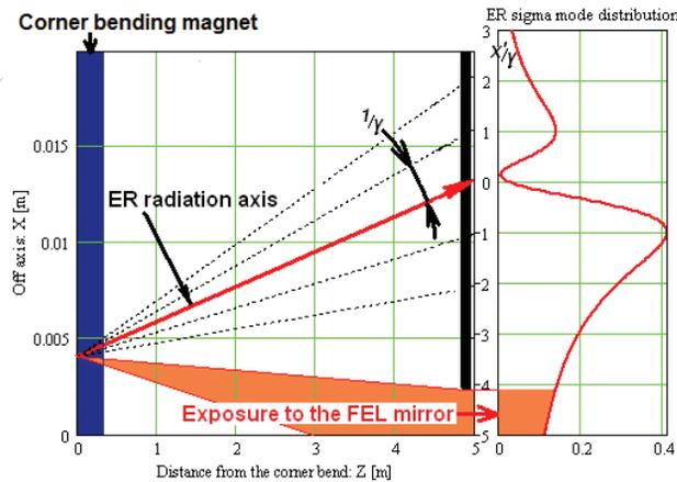
Figure 2: Concept of an orbit bump to protect the FEL mirror from radiation of the corner bending magnet.
