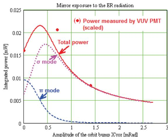
Figure 4: Power of the ER from corner bending magnet integrated in  $\Delta\lambda=170\text{-}290$  nm for the three kicks bump [5].  $E_e=926$  MeV,  $I_e=5$  mA. Amplitude of the soft orbit bump is measured as the total angular kick set for the designated correctors. The measured radiation power using VUV PMT is normalized to the calculated power for  $X'_{cor}=0$ . The measurements for the new orbit bump will be performed and compared with the results of this old bump.
