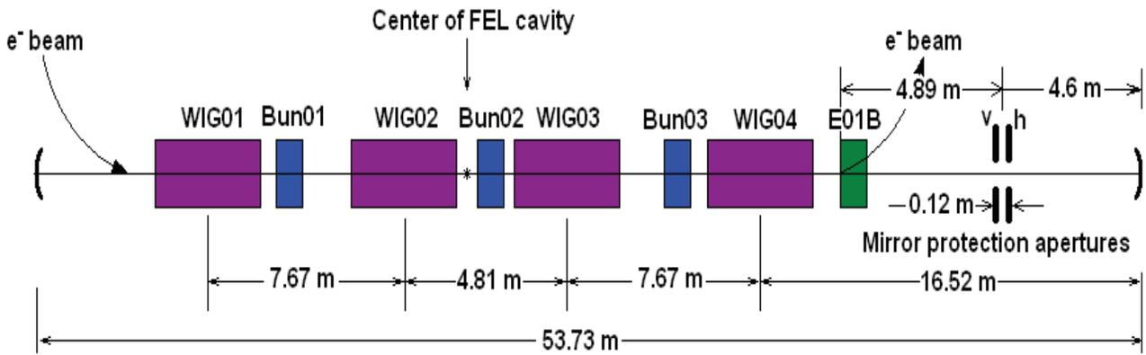
Figure 1: Configuration of the Duke FEL with helical OK5 wigglers.
