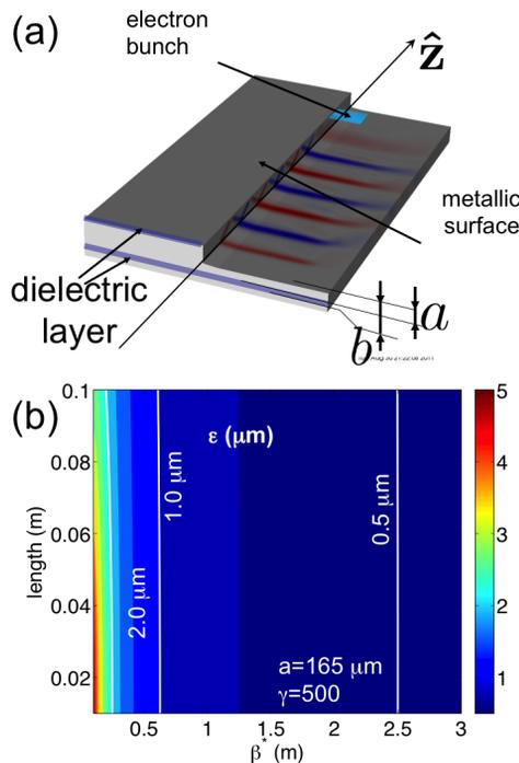
Figure 2: Schematic rendition of the slab-symmetric structure under consideration (a) and required normalized transverse emittance as a function of  $\beta^*$  function and DLW structure length. The DLW inner aperture is taken to be  $a = 165 \mu\text{m}$  and the beam Lorentz factor is  $\gamma = 500$ .
