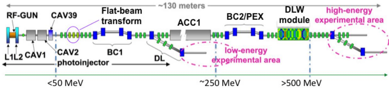
Figure 1: Overview of the Advanced Superconducting Test Accelerator (ASTA). The legend is “L1” “L2” stand for solenoids, “CAV1”, “CAV2”, and “CAV39” correspond to accelerating cavities, “ACC1” to an accelerating module (composed of 8 accelerating cavities), “BC1” and “BC2” to bunch compressors, and “DL” to a dispersionless translating beamline termed as dogleg. “PEX” represents a possible reconfiguration of “BC2” to act as a transverse-to-longitudinal phase space exchanger; see text for details.
