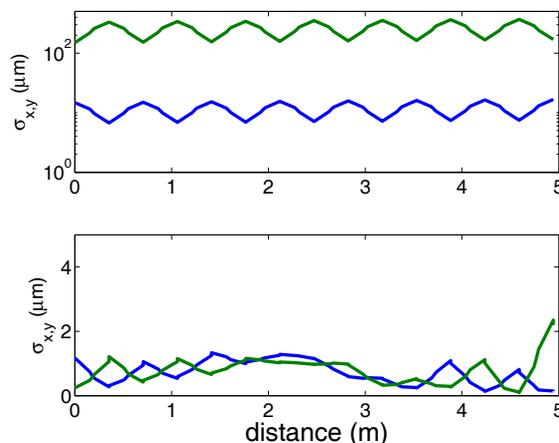
Figure 4: Drive (top) and witness (bottom) bunch rms transverse beam size evolution along a 5-m FODO channel. The two bunches are assumed to have the same initial Courant-Snyder parameters. The witness bunch is accelerated from 250 to 500 MeV while the drive bunch is decelerated from 250 to 225 MeV.
