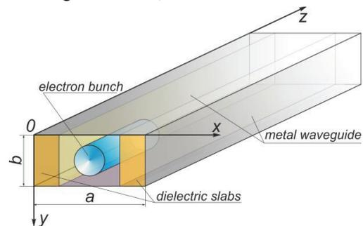
Figure 1: Schematic view of a rectangular dielectric waveguide. Yellow bricks show dielectric slabs, blue cylinder shows electron bunch.
