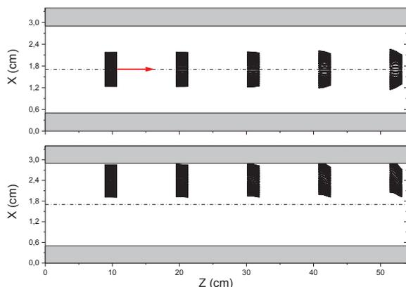
Figure 2: Positions of drive bunch electrons after injection 10<sup>th</sup> bunch of the train: top picture corresponds to on-axis bunch injection; bottom picture corresponds to off-axis injection, offset is 6.8 mm. Drive bunch charge is increased by 10 times in comparison with Tables 1-2 and equal to 3.2 nC. Grey rectangles show dielectric slabs.
