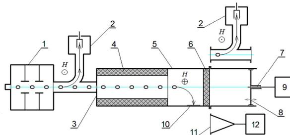
Figure 5: Scheme of the installation: 1-linac, 2-magnetic analyzers, 3-diaphragm, 4-dielectric plates, 5-rectangular copper waveguide, 6-Teflon stub, 7,8-short-circuiting plunger, 9-oscillograph, 10-glass plate, 11-horn antenna, 12-power measurer.
