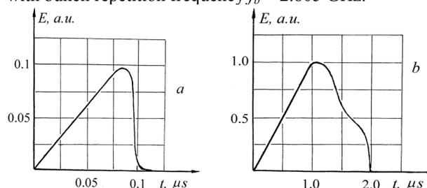
Figure 1: Oscillogram of envelope wakefield excited by a sequences of 300 bunches (a) and 6000 bunches (b).
