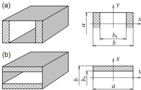
Figure 2: Waveguides with dielectric plates: (a) – along narrow (1st type); (b) – along wide walls of the waveguide (2nd type).
