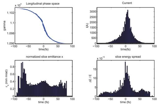
Figure 3: Longitudinal phase space (upper-left), current (upper-right), normalized emittance (lower-left) and energy spread (lower-right) of 100k particles tracked through the extended linac.
