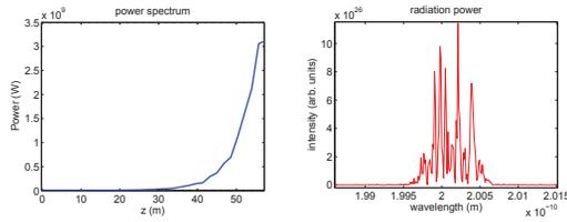
Figure 4: Power along the FEL (left) and wavelength spectrum of the FEL pulse (right).
