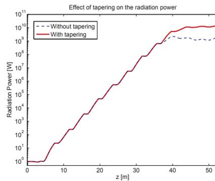
Figure 5: Radiation power as a function of undulator distance for both uniform undulators (blue) and tapered undulators (red).
