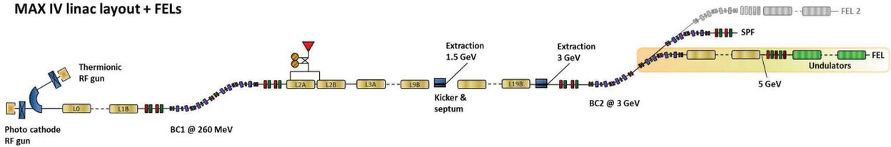
Figure 1: Layout of the MAX IV linac with the extension to 5 GeV and the FEL undulators.
