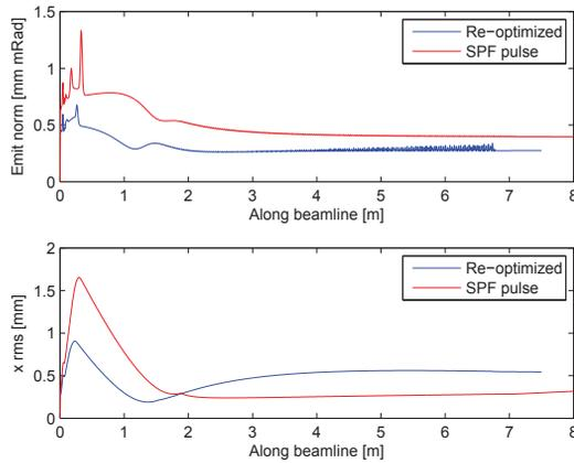
Figure 2: The emittance (top) and the beam size (below) for the SPF optimization (red) and the low emittance, ramped linac field case (blue).
