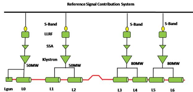
Figure 1: Layout of DCLS linac.
