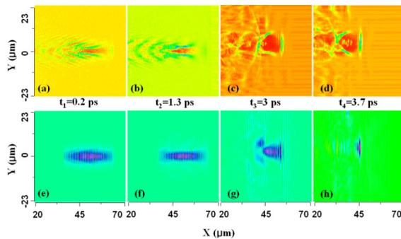
Figure 3: Simulation results: 2D snapshots of plasma density (a-d), and laser pulse evolution (e-h) at time  $t_1 = 0.06$  mm/c (3a, 3e),  $t_2 = 0.4$  mm/c (3b, 3f),  $t_3 = 0.9$  mm/c (3c, 3g) and  $t_4 = 1.1$  mm/c (3d, 3h).
