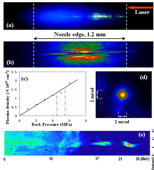
Figure 2: Experiment results: typical top-view and shadow-view images are showed in (a) and (b), respectively. Pressure dependent plasma density is calculated from transmitted light spectrum and presented in (c). Monoenergetic beams can only be generated in backing pressure between the red dashed lines. Electron beam profile obtained on an 18- $\mu$ m-Al foil wrapped phosphor screen and spectra obtained after the dispersive magnet are shown in (d) and (e), respectively.
