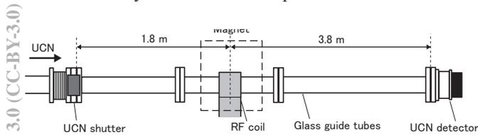
Figure 3: The setup of UCN rebuncher experiments in ILL.
