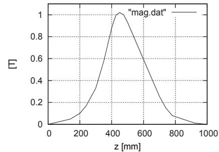
Figure 4: The UCN-transit axial distribution of the magnetic fields strength perpendicular to the axis.
