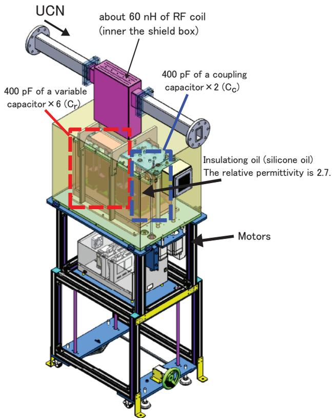
Figure 6: The CAD image of the new UCN rebuncher.
