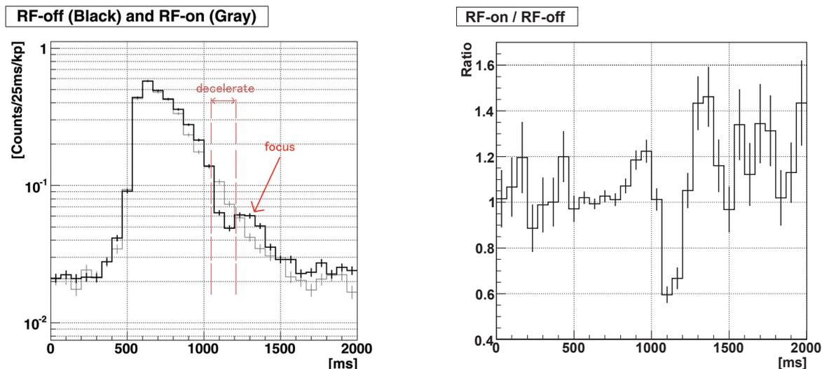
Figure 5: The result of the focusing experiment. (Left) The comparison of Time-of-Flight spectrums with or without the RF-power inputs. (Right) The proportions of the result with the RF-power inputs to without.
