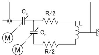
Figure 2: The RF circuits of the UCN rebuncher.
