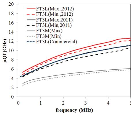
Figure 4: Characteristics of MA cores for J-PARC accelerator use. The FT3M cores (black lines) are currently used for J-PARC. And, FT3L cores in 2011 (bold black lines) are also used in the MR from summer 2012. The recent production (red lines) shows the highest performance. The J-PARC-made cores are even better than the commercial available FT3L cores (blue line) with smaller size. The blue line is overlapping on the bold black line.
