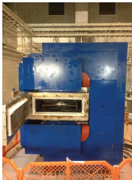
Figure 3: The FT3L core production system using the Kappa magnet. The inner size of the oven is 1.1 m(W) X 0.37 m(H) X 1.4 m(L) to anneal the large size core up to 0.85 m diameter.
