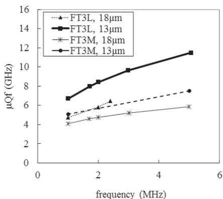
Figure 1: Characteristics of MA cores. The present FT3M core (solid line) with 18 μm layer thickness can be improved by the FT3L with 13 μm thickness (bold line).
