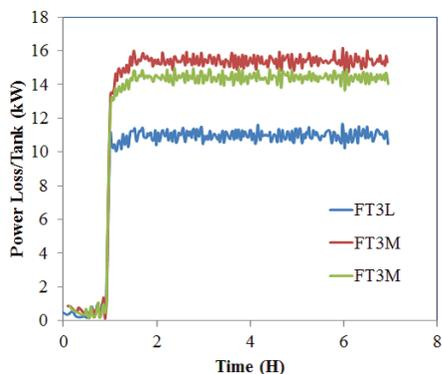
Figure 2: Power consumption in half cavity cell calculated by temperature rise of cooling water during machine operation. Because of the higher impedance compared to the other cavities, the temperature rise of the FT3L cavity cell is much lower than that of the other FT3M cavity cells.
