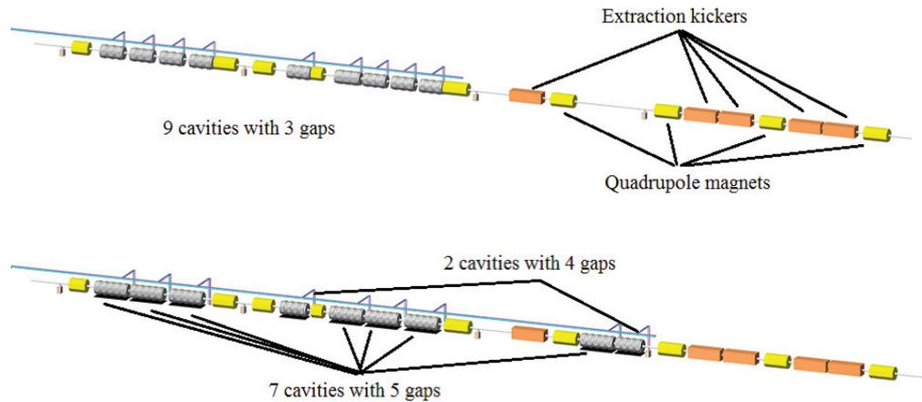
Figure 5: Upgrade scenario of J-PARC MR cavities. The present cavities (upper) will be replaced by the FT3L cavities (lower) in 2014-2016. The total RF voltage will become 560 kV providing enough margin as the required RF voltage for 1 Hz operation is 440 kV according to a simulation.
