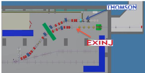
Figure 2: Details of the SPARC\_LAB facility showing all the electron beam lines, downstream the injector from right to left: FEL undulators, THz source, Plasma Acceleration experiments, Thomson backscattering source.
