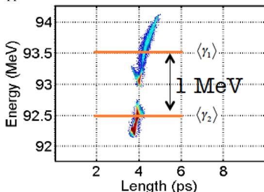
Figure 5: Measured longitudinal phase space of the double electron pulse showing the time overlapping and the energy separation of the two bunches.
