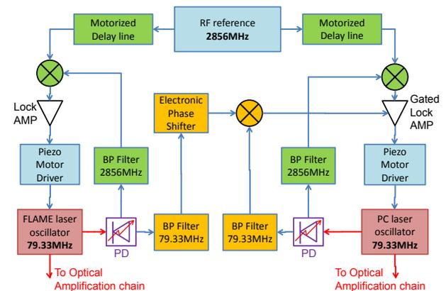
Figure 4: Sketch of the lasers synchronization scheme used in the Thomson scattering experiment.
