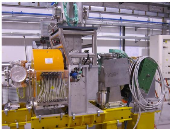
Figure 3: The Thomson scattering interaction chamber.
