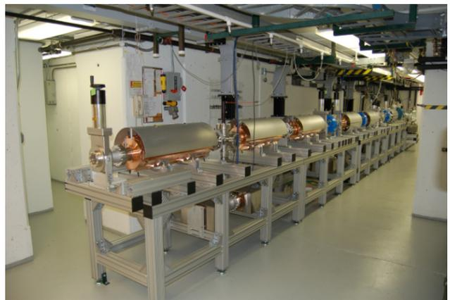
Figure 1: The new linac tanks installed in the AWA bunker. The RF conditioning of these structures will be initiated shortly (June 2013).
