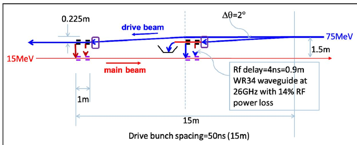
Figure 3: Schematic of the proof of principle experiment to demonstrate staging at AWA. Each stage has two decelerating structures and their corresponding accelerating structures. Correct timing of the RF pulses is obtained by adding appropriate delays to the waveguides connecting the structures
