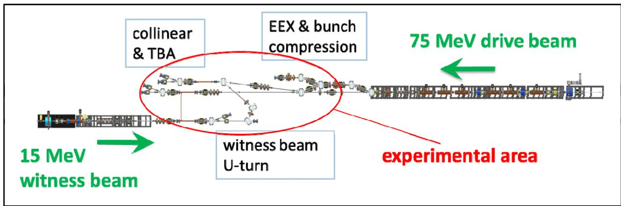
Figure 2: Schematic of the AWA beamlines, showing the Drive Beamline, the Witness Beamline and the beamline switchyard where the various experiments will take place.
