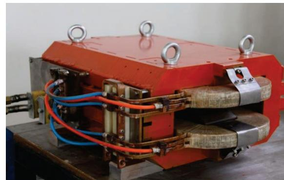
Figure 2: ILSF H-type dipole magnet.
