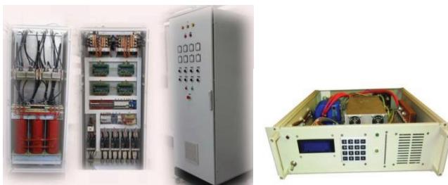
Figure 4. Two prototype power supplies of different rating designed and constructed at ILSF R&D lab.
