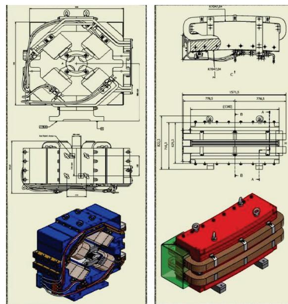
Figure 3: Under construction ILSF storage ring quadrupole magnet (left) and C-type dipole magnet (right).
