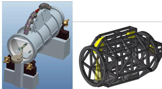
Figure 5: Design studies for iso-centric and super-conducting carbon ion gantries. At NIRS/HIMAC (left) the planned 3T result in a radius of 5.5m whereas the concept presented by IBA/CEA (right) is based on 5.4T magnet design allowing for a very compact radius of 4m only.
