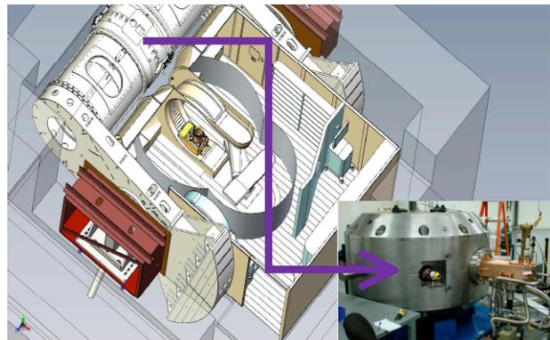
Figure 1: The Mevion S250® Proton Therapy System is based on a 9T, Nb3Sn, synchro-cyclotron that rotates closely around the patient.
