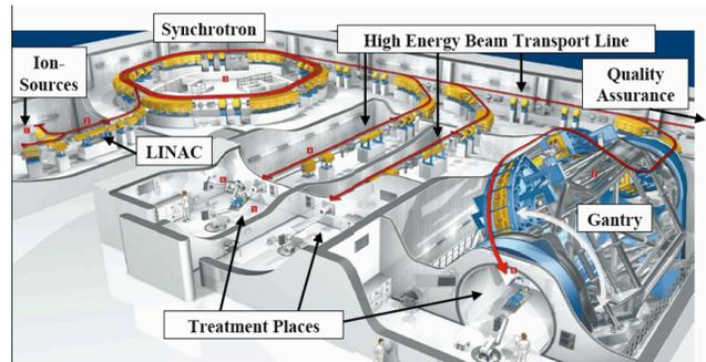
Figure 3: The Heidelberg Ion Beam Therapy Centre HIT.
