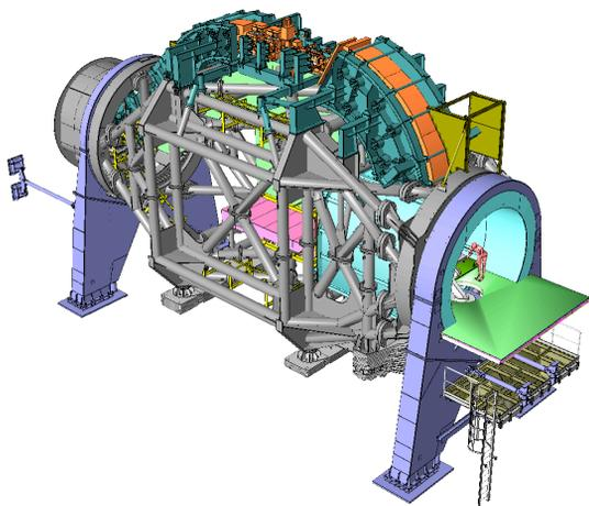
Figure 4: HIT's worldwide first iso-centric scanning ion gantry. This unique device was realized in a cooperation of GSI, Darmstadt, Siemens Medical Solutions, MT Mechatronics and HIT, Heidelberg.
