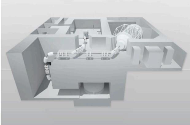
Figure 2: IBA's Proteus Nano® two-room solution aims at a very compact footprint by distributing the particle accelerator technology over two levels.
