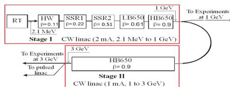
Figure 2: Acceleration scheme for various stages.
