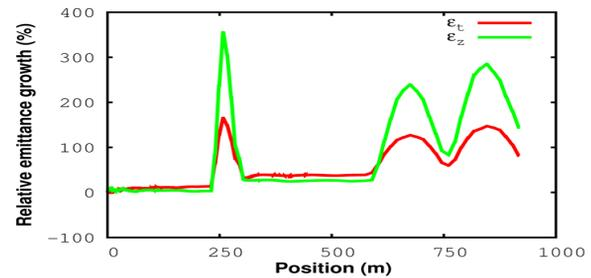
Figure 4: Relative emittance growth along the linac in longitudinal (green) and transverse (red) plane.
