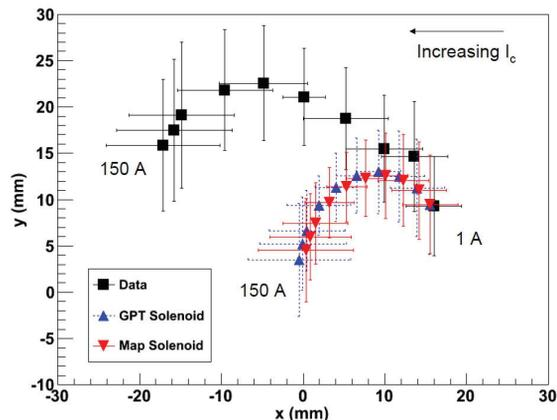
Figure 2: LEBT beam centre behaviour in simulation and measurement.
