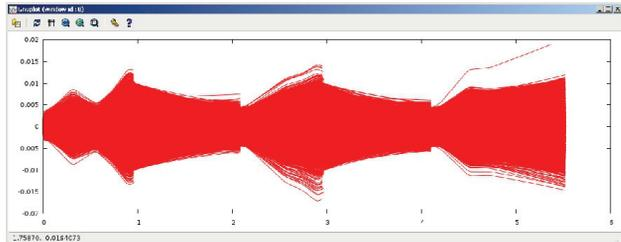
Figure 5: Vertical beam envelope in the alternative MEFT.
