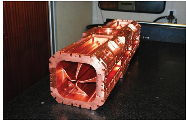
Figure 3: Test assembly of RFQ section 1.
