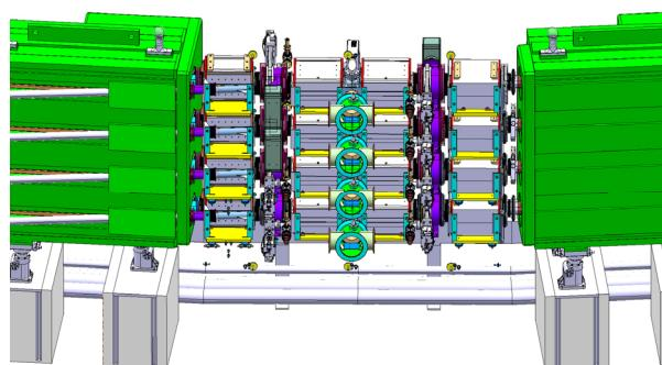
Figure 3: Injection period modified for injection of 160 MeV H<sup>-</sup> ions from Linac4. In-between two main dipole magnets there is a system of 4 chicane dipoles, with the stripping foil unit in its center. Every ring is equipped with its proper injection hardware.
