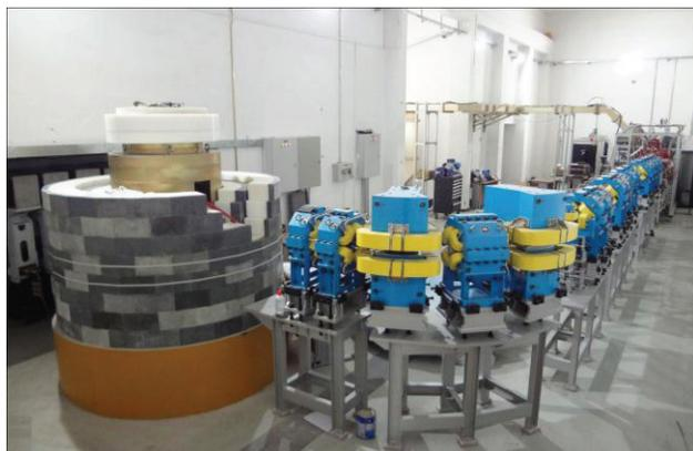
Figure 5: target station and HEBT
