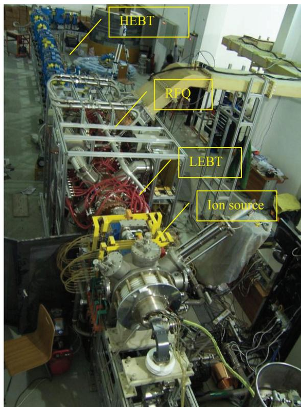
Figure 1: photograph of CPHS linac from IS to HEBT
