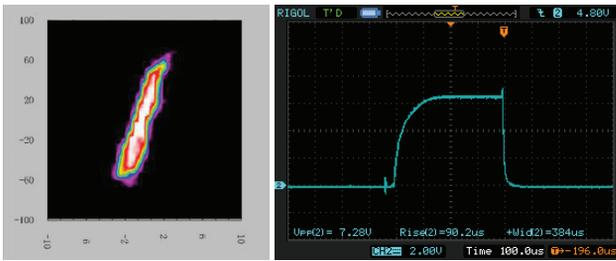
Figure 2: emittance (left) and current (right) measured at the exit of LEBT
