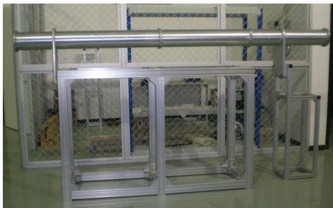
Figure 6: TOF tube for neutron imaging
