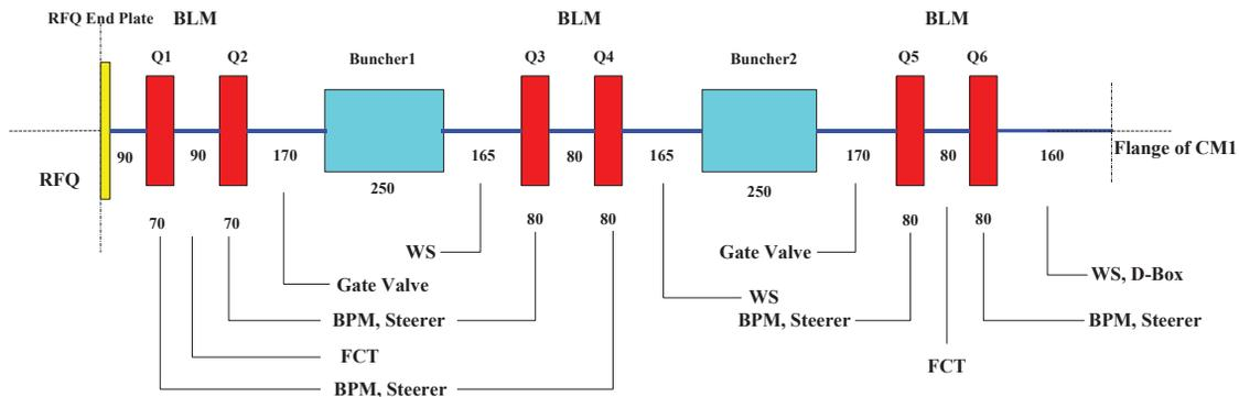
Figure 4: Schematic of the MEBT1 for Injector Scheme.
