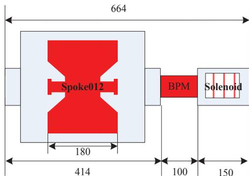
Figure 5: Layout of one focusing period in Injector Scheme-I.
