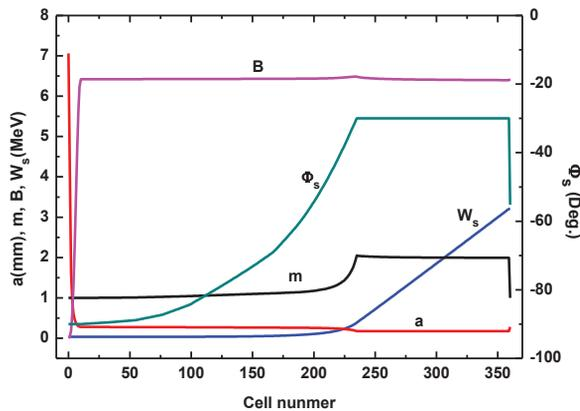
Figure 3: Main parameter variation with cell number, where a stands for the minimum bore radius, m modulation factor, B focusing factor, W synchronous energy and  $\Phi_s$  synchronous phase.
