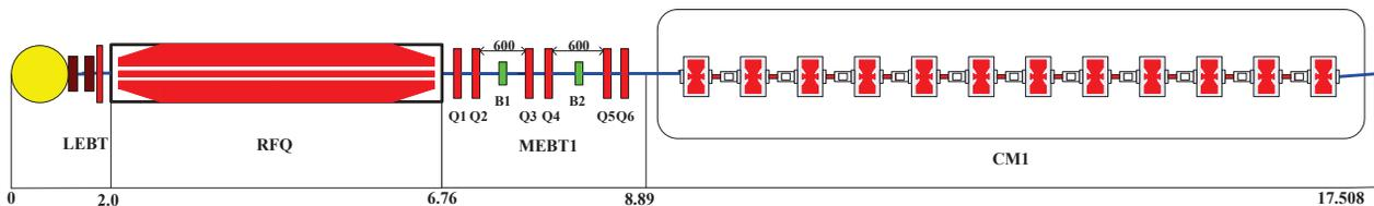
Figure 2: The schematic layout of the Injector Scheme-I.
