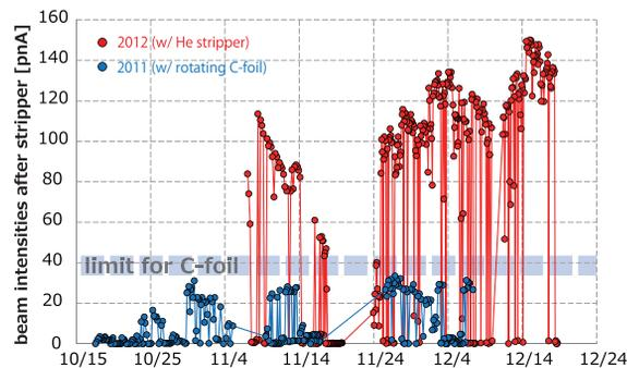
Figure 4: The intensity of the beam through the first stripper in 2011 and 2012.
