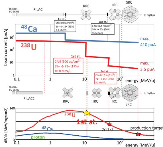
Figure 1: The acceleration scheme of uranium and calcium ions in 2011 at the RIBF. The energy dependence of dE/dx for  $^{238}\text{U}$ ,  $^{48}\text{Ca}$  and proton are also shown at the bottom of the figure.
