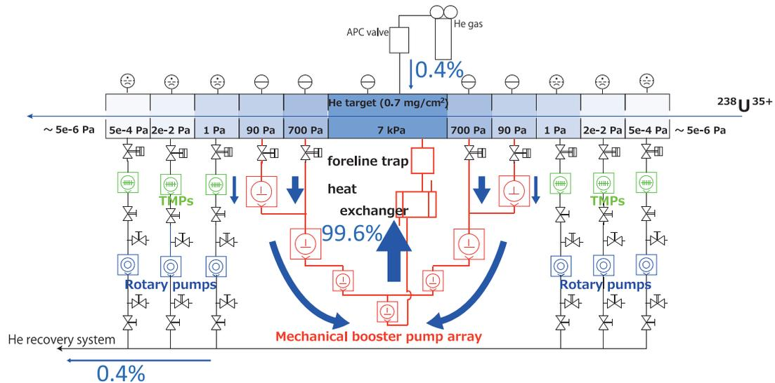
Figure 2: Schematic of the He recirculating system. The multistage MBP array consists of 7 MBPs.
