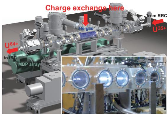
Figure 3: Cross sectional view of the He gas stripper and picture of glowing 1- $\mu A$  uranium beams.
