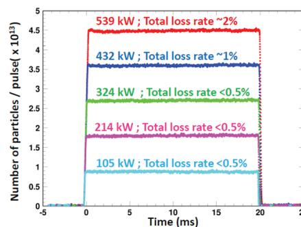
Figure 2: Signal of the beam current monitor (DCCT) and total beam loss rate in the case of the beam power form 105 kW equivalent to 539 kW equivalent. Horizontal is time and vertical is number of particles per pulse. The beam power was controlled by the pulse length of the injection beam from the Linac. The pulse length was changed form 100 micro-sec to 500 micro-sec.
