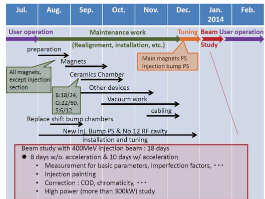
Figure 4: Schedule of maintenance and 400 MeV beam injection upgrade in the RCS in this maintenance period.
