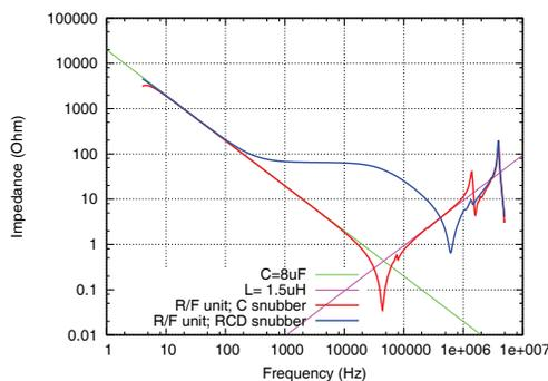
Figure 4: The internal impedance of the rise-fall unit. Temporary, small DC power supplies to charge the main capacitor were removed.
