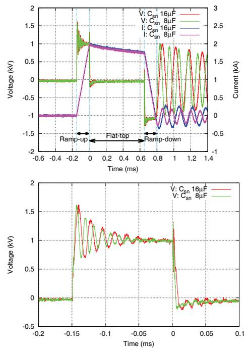
Figure 1: The output voltage and current waveform of single rise-fall unit. Lower plot is zoom of the output voltage during the current ramp-up period. The dependence of snubber capacitance is observed.
