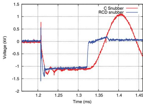
Figure 3: An output voltage comparison with C-snubber or RCD-snubber during the current ramp-down period.
