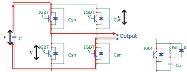
Figure 2: The circuit diagram model of the unit. There are four IGBTs, switching device, and its snubber circuit to prevent over voltage on IGBT. The left-side C is a main capacitor (24 mF) and it can be considered as DC battery during a few ms. Right one is a RCD snubber circuit.
