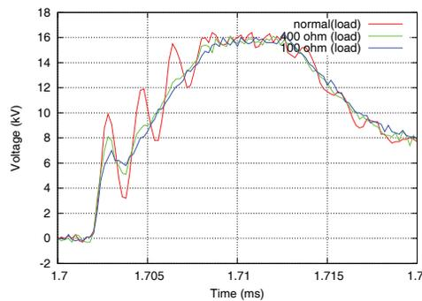
Figure 5: The output current and voltage pattern of one bank. Higher frequency ringing (400 kHz) is damped by adding resistor parallel to the output port. Lower plot is zoom of upper plot.
