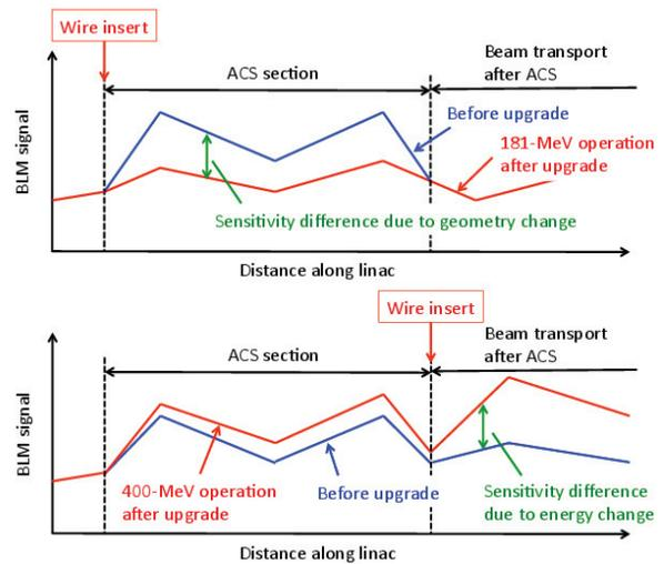
Figure 1: Schematic for the proposed BLM calibration for the effect of geometry difference (top) and energy difference (bottom).
