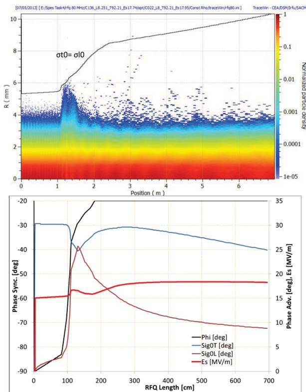
Figure 2: In the upper part the Radial density along the RFQ, in the lower part the phase advance, synchronous phase and Surface Field along the RFQ.
