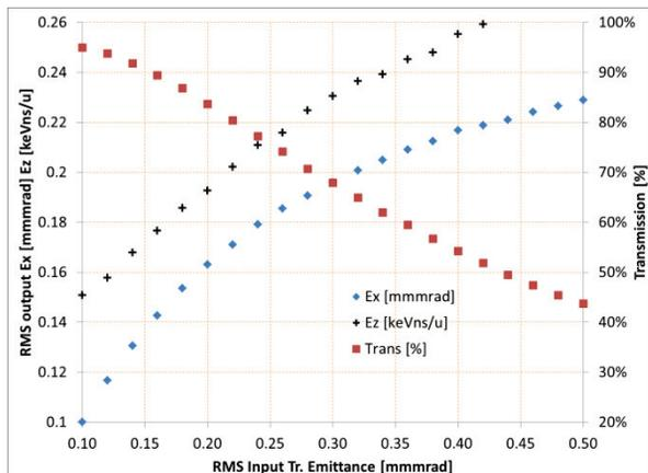
Figure 3: Output emittances as function of input emittance.
