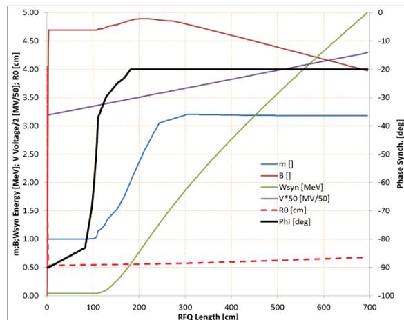
Figure 1: The main RFQ parameters vs. length.
