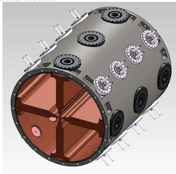
Figure 4: Mechanical layout of the RFQ tank module of about 1 meter.
