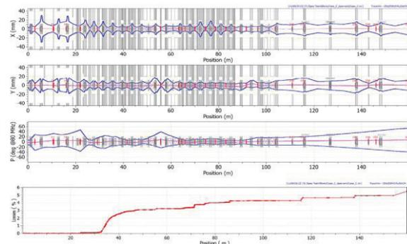
Figure 7: Multiparticles envelopes of the ALPI and losses, with the beam coming out from the SPES RFQ, from left to right.
