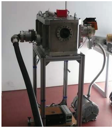
Figure 3: Prototype in cavity tank and its 1 5 / 8 inch coaxial transmission line.
