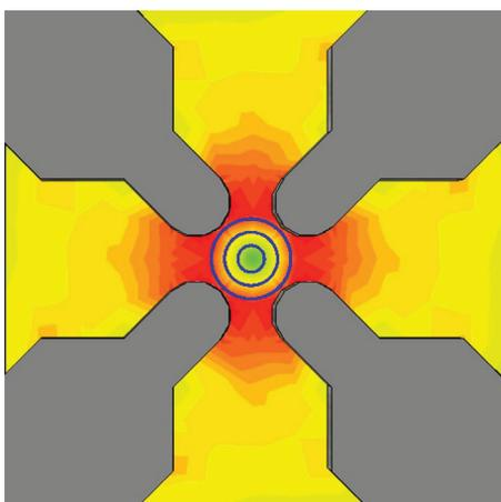
Figure 3: View along the beam axis with a contour color plot of the absolute electric field values. One can see qualitatively that all vanes are on the same absolute field level.
