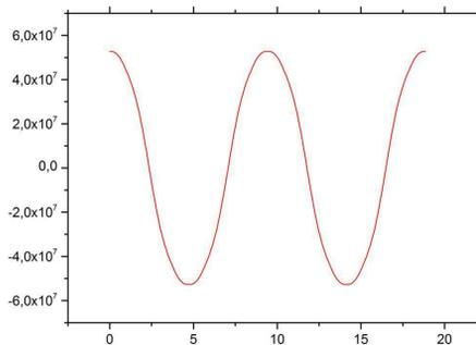
Figure 4: Plot of the absolute electric field along a curve around the beam axis.
