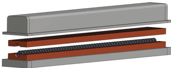
Figure 6: 3-D view of the complete cavity demonstrating the assembling concept.
