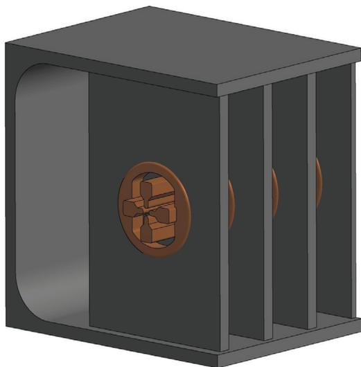
Figure 1: 3D-Sketch of a ladder RFQ, consisting of the tank, stems, carrier rings and mini-anes.
