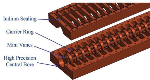
Figure 5: 3-D view of the copper structure showing the components and the assembly concept.
