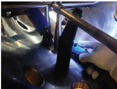
Figure 7: The camera assisted welding operations.
