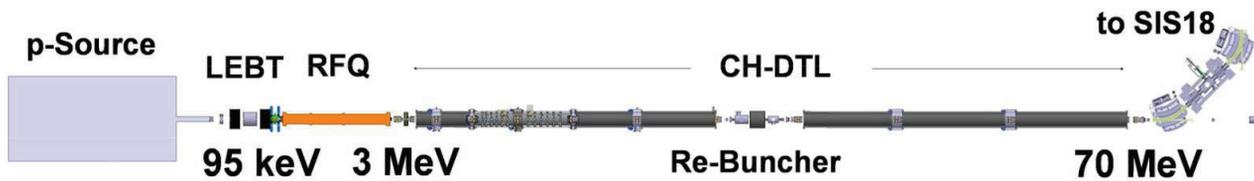
Figure 1: The schematic layout of the FAIR proton linac.
