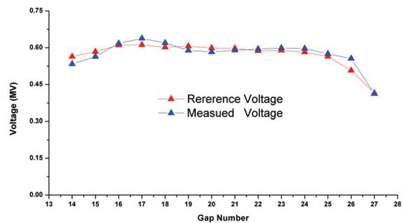
Figure 4: The field distribution in the first CH section.
