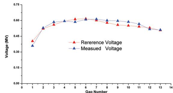
Figure 5: The field distribution in the second CH section.
