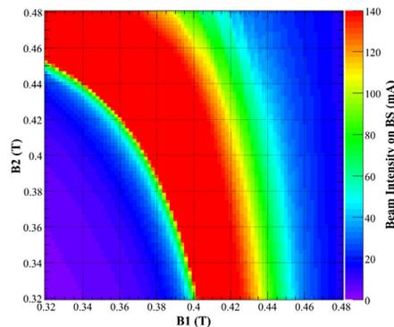
Figure 3: Simulation results: beam intensity at the end of the LEBT as a function of solenoids magnetic field.
