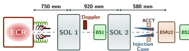
Figure 1: Scheme of the LIPAC injector.
