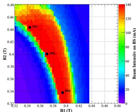
Figure 2: Experimental results: beam intensity at the end of the LEBT as a function of solenoids magnetic field.
