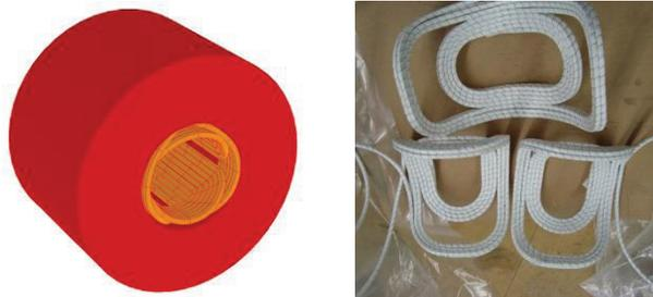
Fig. 3: Principle of H/V steerers located inside solenoid (left) and picture of steerers coils before assembly (right)
