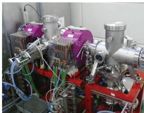
Fig. 4: View of the Injector LEBT before connection of all the water cooling circuits
