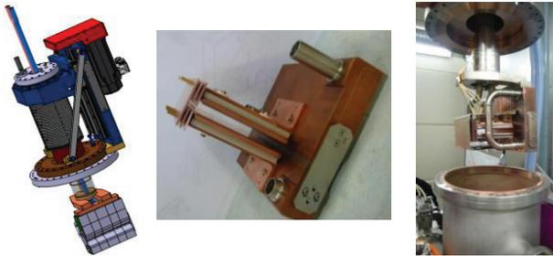
Fig. 5: LIPAc injector emittancemeter
