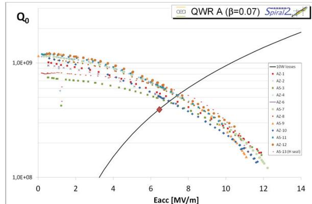
Figure 1:  $Q_0$  vs.  $E_{acc}$  curves of  $\beta=0.07$  cavities.
