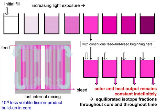
Figure 2: Concept of operating with equal fill and removal rates to maintain a constant reactor performance.
