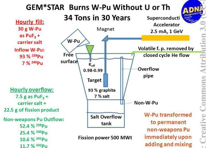
Figure 3: A GEM\*STAR unit to generate heat by burning W-Pu while making remnants unusable for nuclear weapons. Four GEM\*STAR units will treat 34 tonnes of W-Pu to provide 80 billion gallons of diesel fuel, which is about what the DOD needs for the next 30 years.
