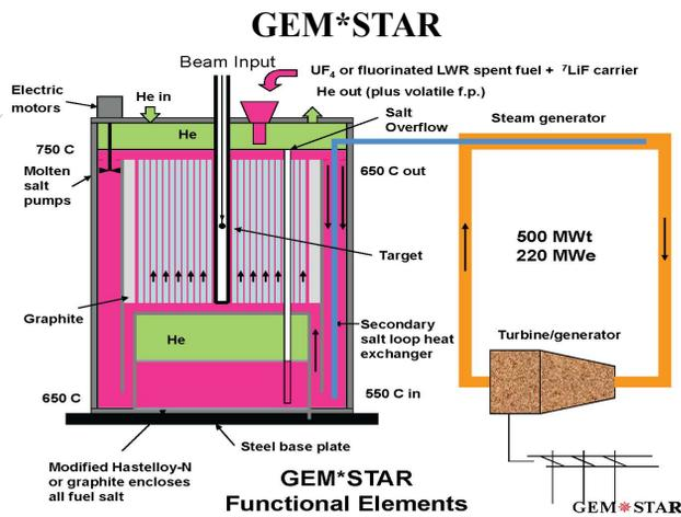
Figure 1: Conceptual arrangement of a GEM\*STAR reactor unit configured to produce electricity. To produce diesel fuel, the secondary salt loop heats CH<sub>2</sub> and H<sub>2</sub>O to produce CO and H<sub>2</sub> for the Fischer-Tropsch process.
