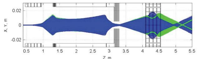
Figure 1: Particle trajectories from solenoid through acceleration section.
