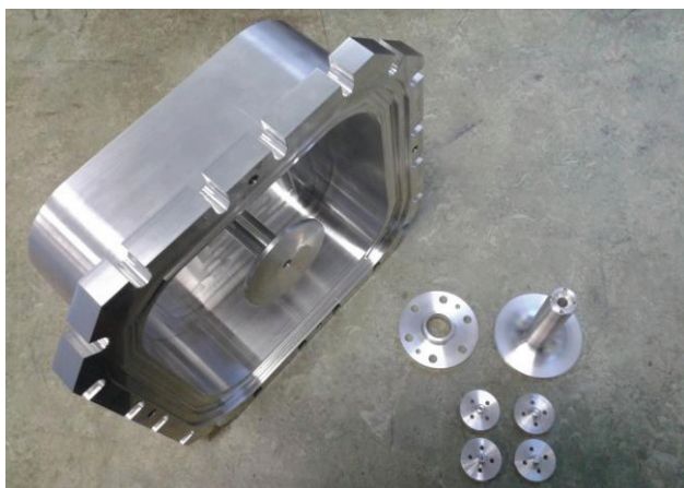
Figure 3: One bead-pull test end flange assembly.
