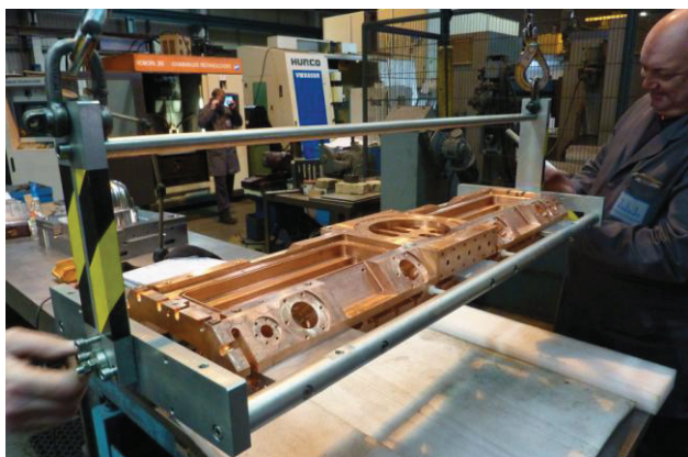
Figure 2: RFQ section 1 in the lifting frame.
