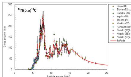
Figure 1: Cross section for <sup>11</sup>C production, from [3]
